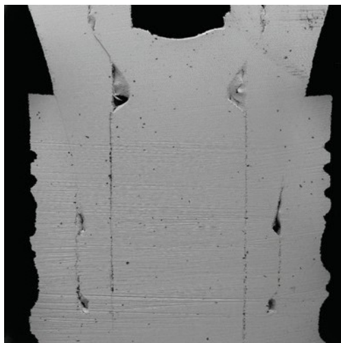
Fig. 13: Abutment fitting for a BioniQ® Implant (SEM image, 100x).
