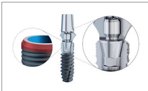
Fig 3b Q-lock connection between the intraosseous part of the implant and the abutment (anti-rotation element together with both the conical tapered and tube-in-tube connection). The modified osteoconductive surface of moderate roughness is shown as a red collar on the implant neck.
